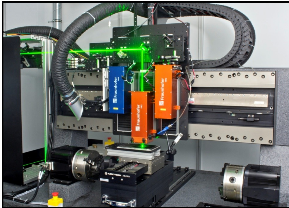
Fig. 9. Large area DLIP system for processing 2D and 3D parts.
