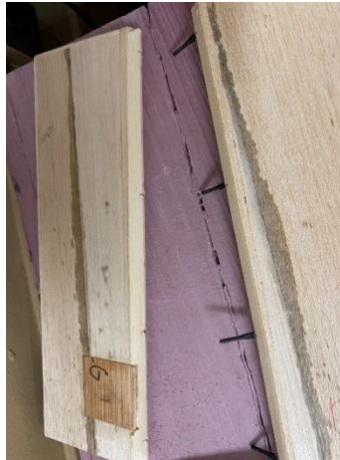
Figure 9.8: Balsa supports along the hinge line between the wing and aileron, showing the hinging for the aileron and the support area for control horn.
