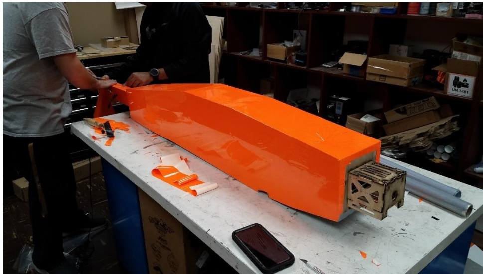
Figure 9.13: Covering the Fuselage with MonoKote
