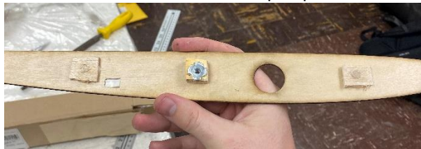
Figure 9.7: Components along the inside of the root cap including alignment pins and locking bolt for the wing screw.
