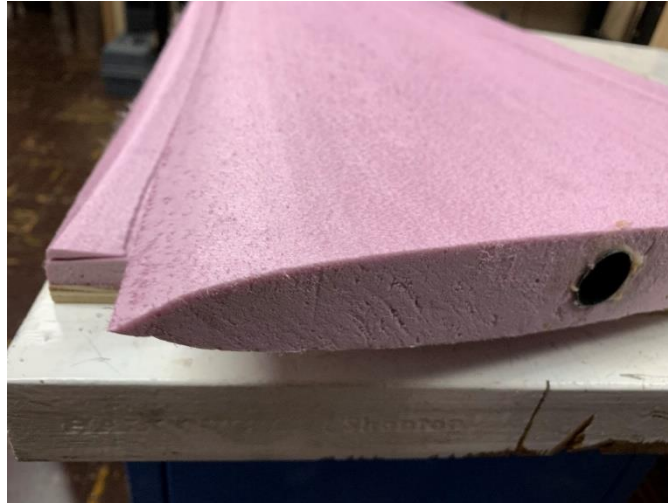
Figure 9.5: Foam core cut into the correct shape by the hotwire cutter and phenolic tube installed into the core.
