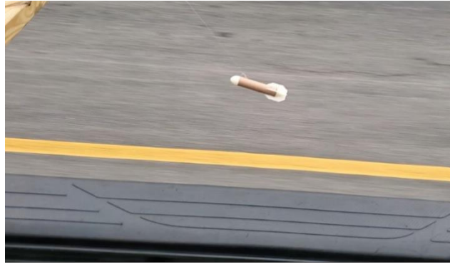
Figure 8.5: Aerodynamic stability test of sensor with non-conformal fins
