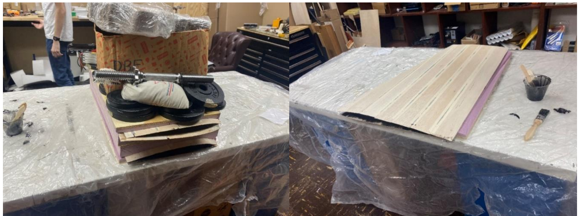
Figure 9.6: Skinning process for foam core wings.
