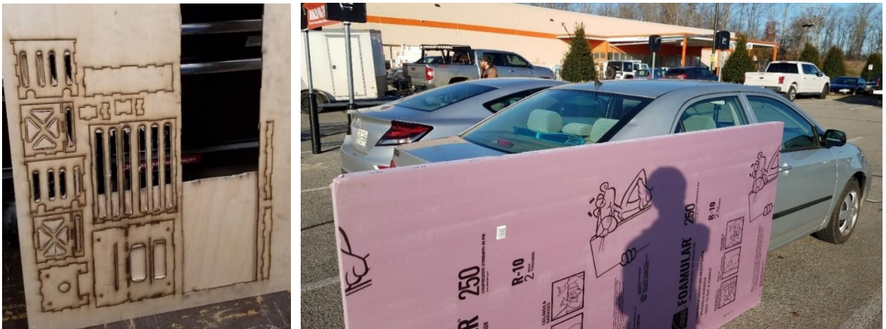
Figure 9.4: Main materials used for construction, LitePly Plywood (left) and insulation foam (right).
