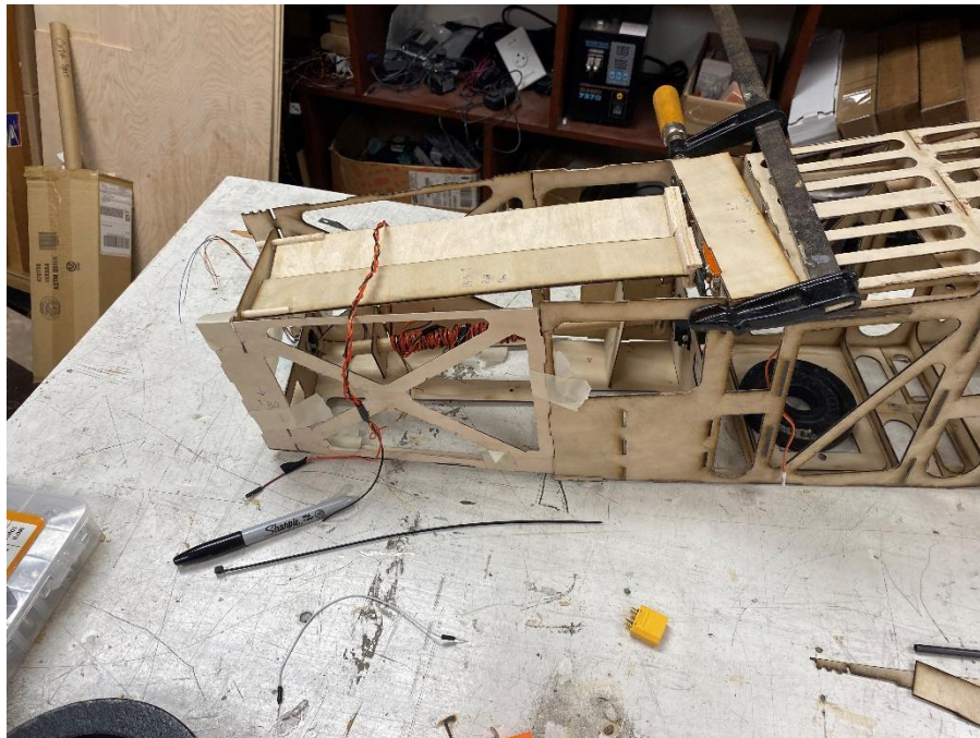
Figure 9.11: Deployment System Construction
