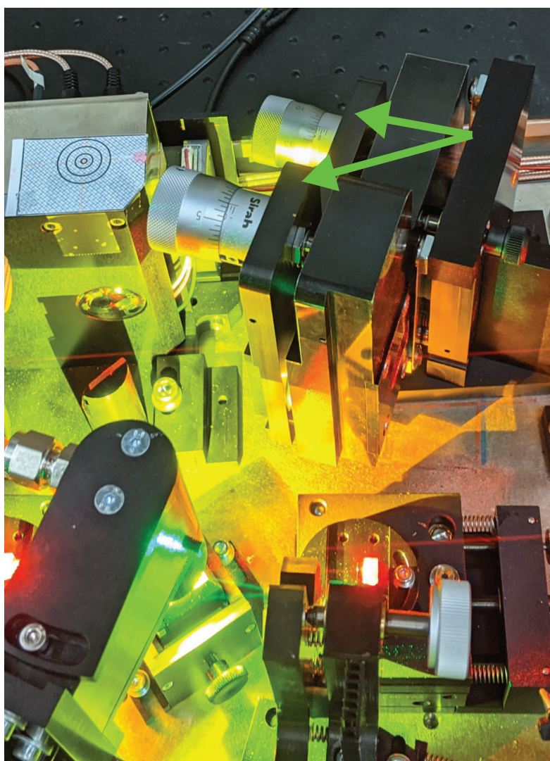
FIGURE B.3: Vertical and Horizontal adjustment knobs for the thick etalon.
