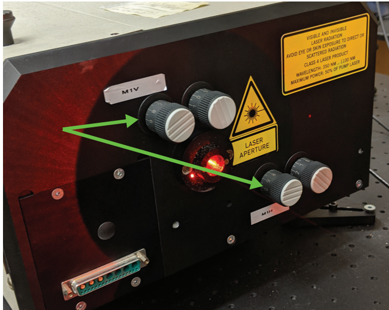
FIGURE B.1: Vertical and Horizontal adjustment knobs for the output couple (M1).
