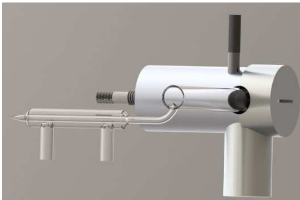
FIGURE 4.6: Iodine plasma source used in this work. A quartz cell designed with a chilling finger is sealed with a static pressure of < 10^{-4} Torr. The cell is inserted into an Evenson microwave cavity that is responsible for maintaining the plasma after ignition.
