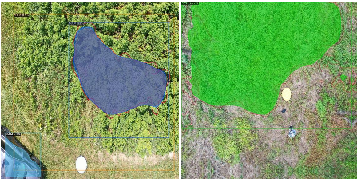
Figure 5.8: Augmented dataset's (section 4.3) Mask R-CNN results with Softmax threshold = 0.5. With this threshold, we have false alarms such as car detection.
