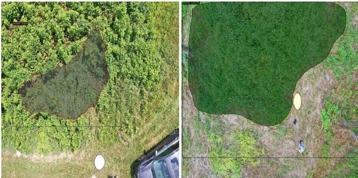
Figure 5.7: Augmented dataset's (section 4.3) Mask R-CNN results with Softmax threshold = 0.9. The number on the top of the bounding box is the probability of MAM's presence.
