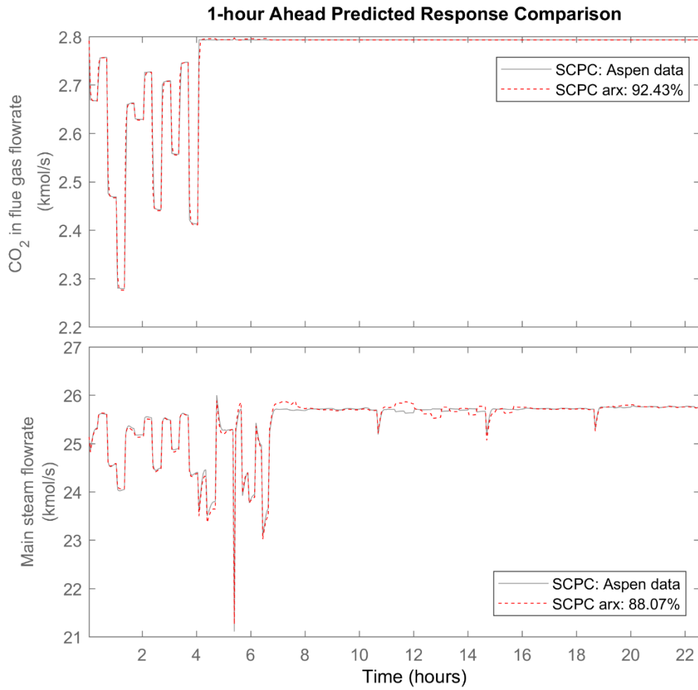
Figure 4.3. Comparison between 1-hour ahead model prediction with data from high-fidelity Aspen model – SCPC linear ARX
