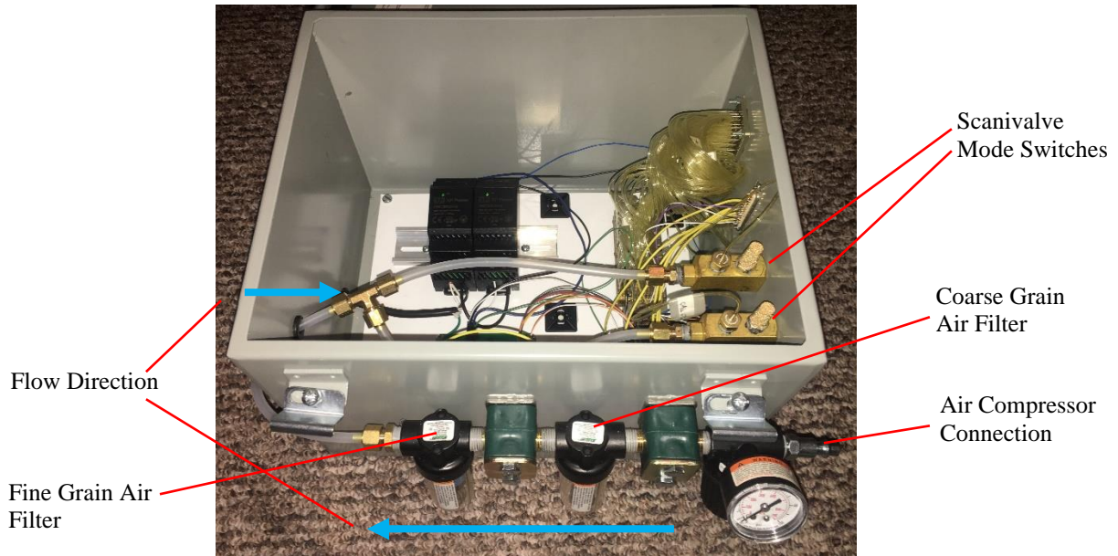
Figure 4.8: Scanivalve housing box, open.
