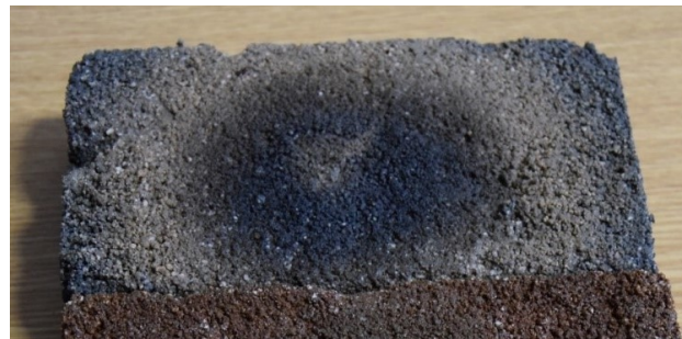
FIGURE 8. H-cement mortar after the experiment and after fast cooling in water.
