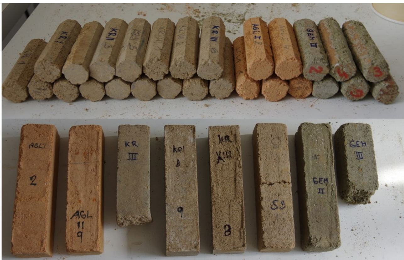
FIGURE 3. Specimens with different type of clay as a binder.
