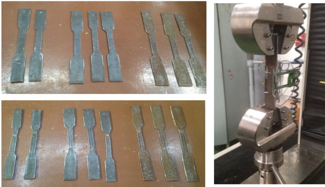
FIGURE 4. Coupon tests specimens and scheme of loading.
