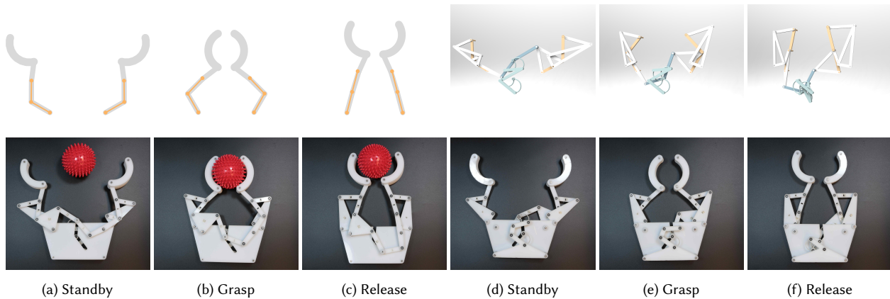
Fig. 15. GRIPPER poses result (top row: rendered; bottom row: physical artifact). The three poses are shown from the front and the back.
