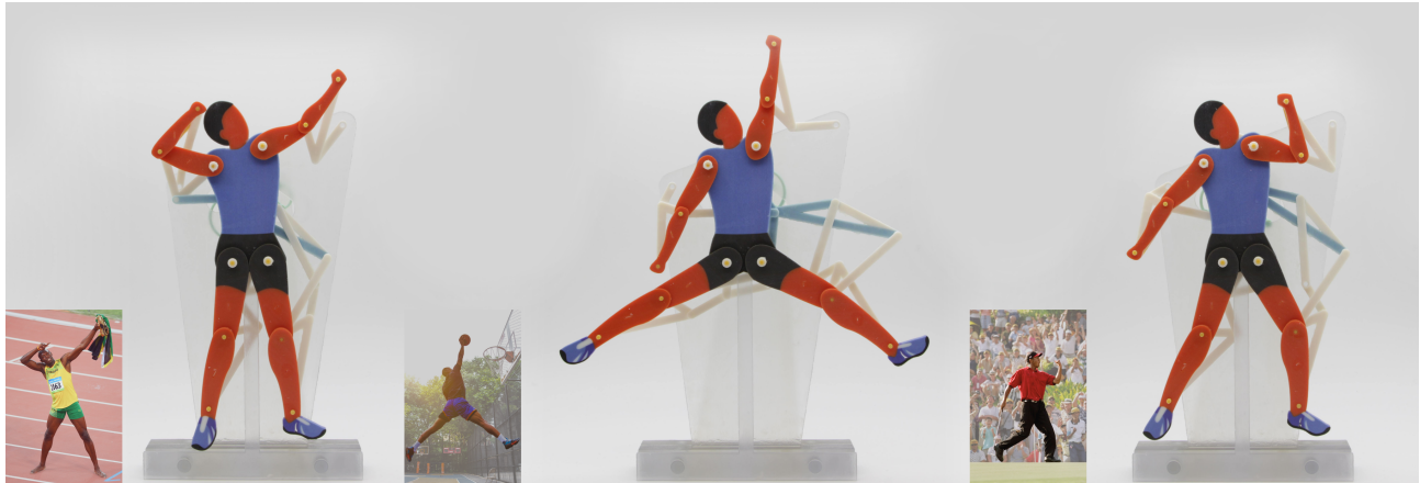
Fig. 1. The optimization-based design tool that we have introduced enables the computation of multistable compliant structures that can, e.g., be used to pose physical figurines.
