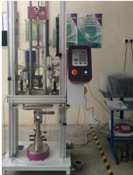
Figure 1: An experimental set-up for drop weight impact test using an INSTRON CEAST 9340 machine
