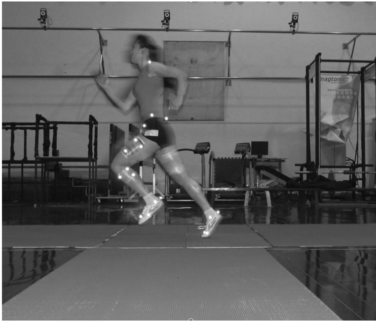
Figure 1. A synthetic rubber track was placed on the laboratory floor and the force platform.
