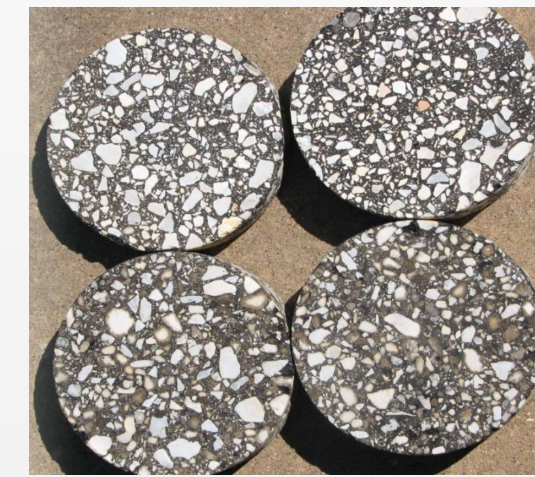
Hamburg Wheel Test- After 1 Year
