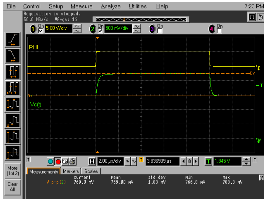
Figure 3-9 Transient scope view of V_c when irradiance = 25\ \mu\text{W}/\text{cm}^2 .
