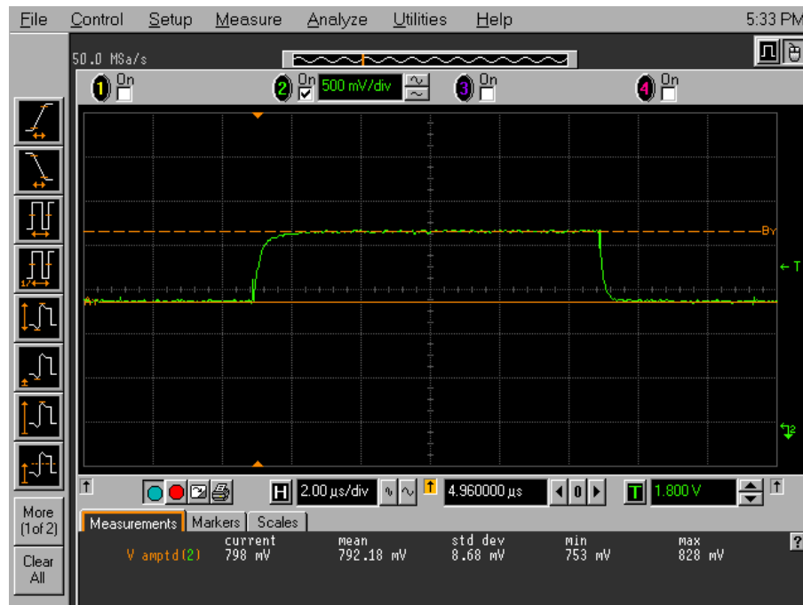
Figure 3-3 Column output voltage V_C when V_B=2.5\text{V} .
