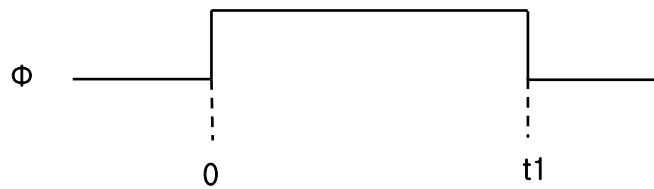
Figure 2-4 Scheme of clock signal \phi for SRL pixel operation.
