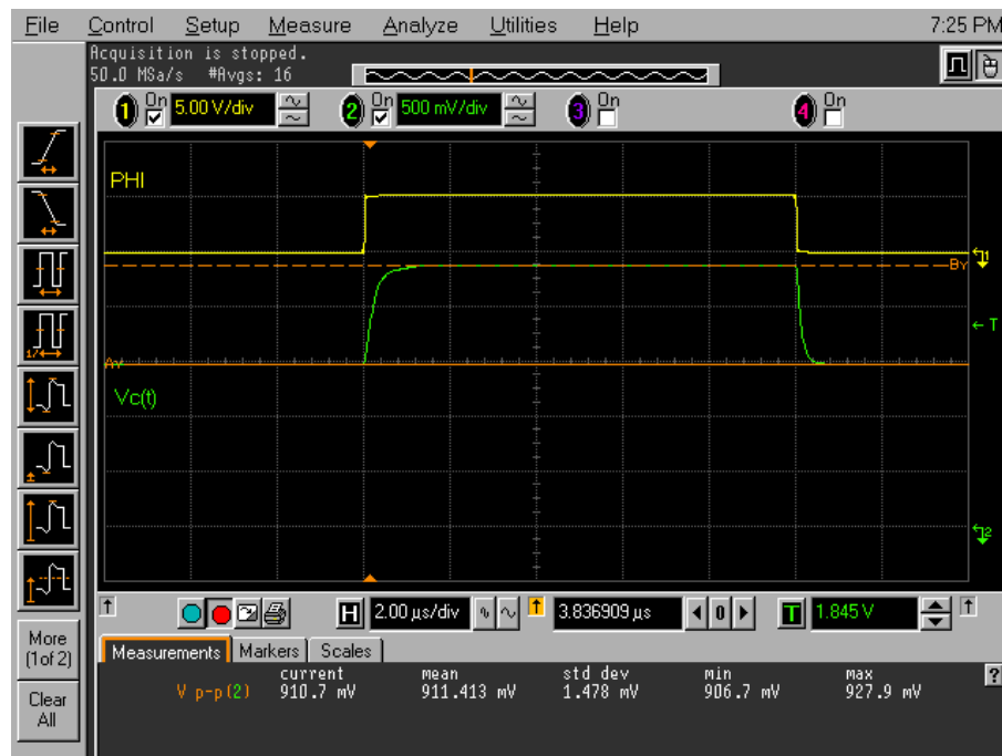
Figure 3-10 Transient scope view of V_c when irradiance = 250\mu\text{W}/\text{cm}^2 .
