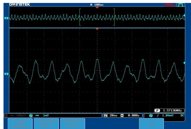
Fig.5 First stage of OPAMP output
