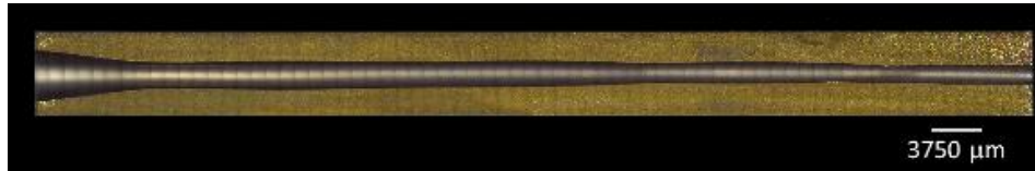
Fig. 9 Exemplification view of the internal surface of the worn focusing tube
