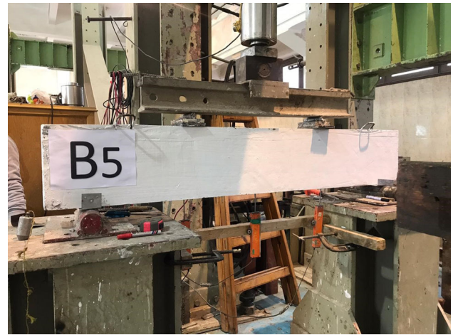
Fig. 4 Test setup for a typical beam
