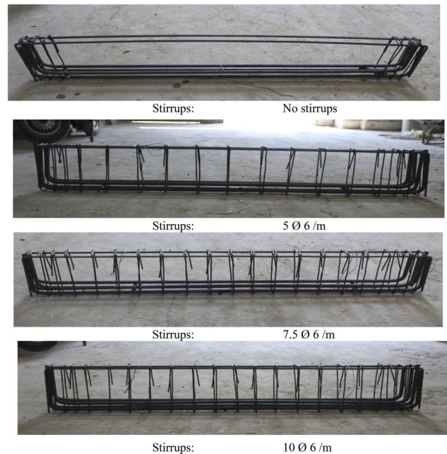
Fig. 2 Steel reinforcement cages for typical specimens
