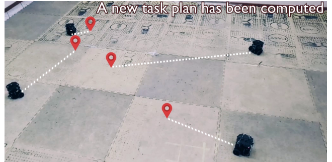
Fig. 4. Snapshot from the dynamic task assignment experiment. Robots move in order to reach their designed tasks (red markers).
