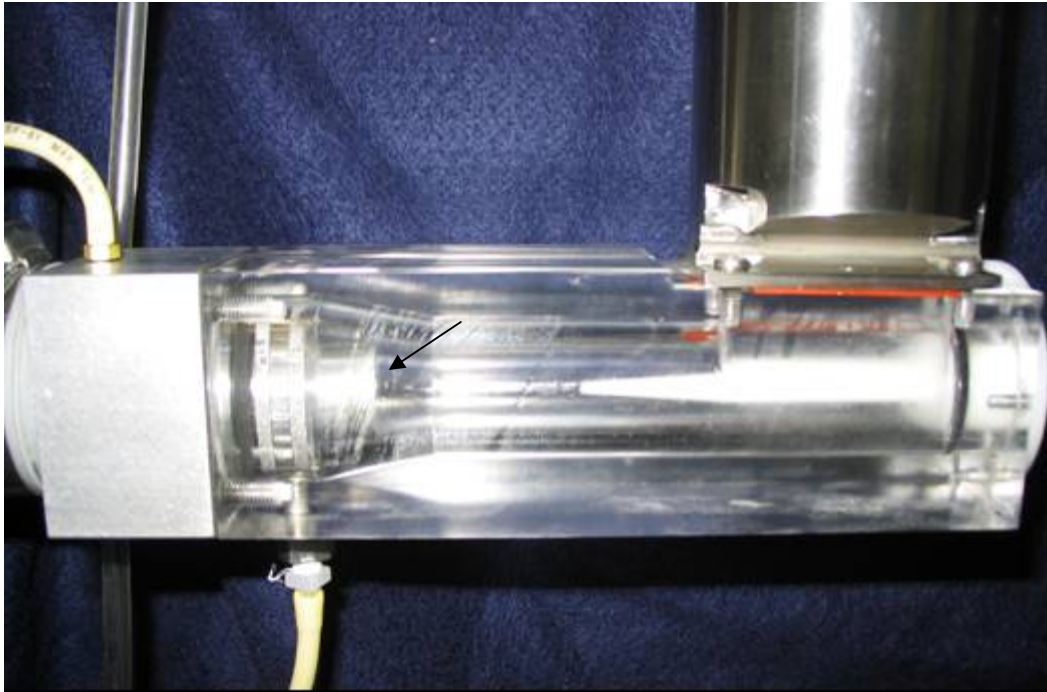
Figure 11. Acrylic AAC with outlet skimmer modeled after White-type cyclone (ca. 2003). The arrow indicates the recirculation area.
