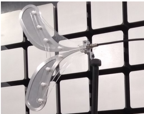
Fig. 1. 530 mm×760 mm (L× H) Coplanar Vivaldi with weight reduced blades and acrylic support structure under test in anechoic chamber
