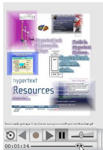
FIG. 3. Preview with the Jog-Shuttle History Slider. The image shows the snapshot of the preview window displayed by combinFormation when the user goes back in the timeline in an information space created by giving the search term “hypertext”. [Kerne and Interface Ecology Lab 2004]
