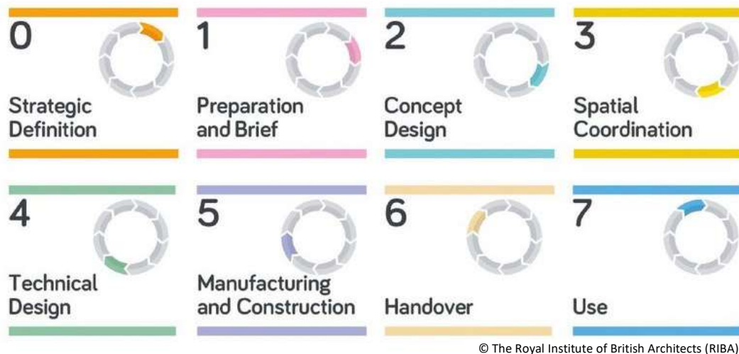
Figure 7.3 – Stages of RIBA Plan of Work 2020 (RIBA, no date, cited in Sinclair, 2019).
