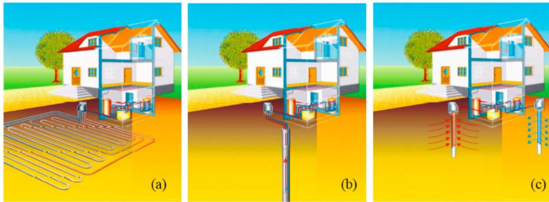
Figure 2.5 – Ground Source Heat Pump (GSHP) system set ups. (a) horizontal closed loop, (b) vertical closed loop, (c) vertical open loop (Bundesverband Wärmepumpe (BWP), 2009, cited in Rodrigo-Harri et al., 2010).
