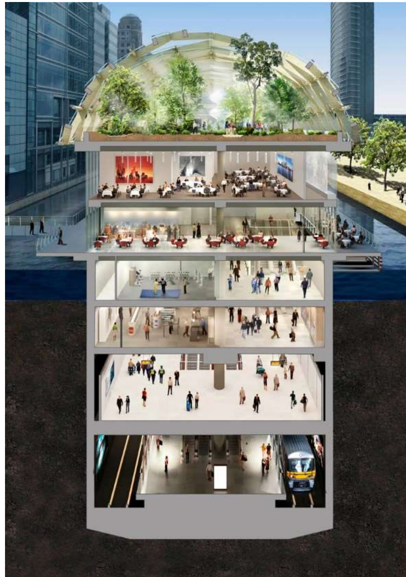
Figure 6.1 – Cross-sectional architects impression of Canary Wharf Crossrail Station (Crossrail Ltd, no date).
