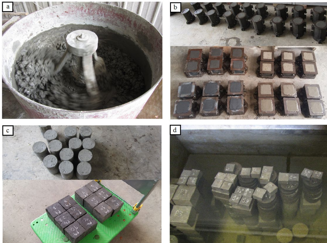
221 Figure 3: Concrete specimens (a) mixing, (b) casting, (c) demoulding and (d) 222 curing
