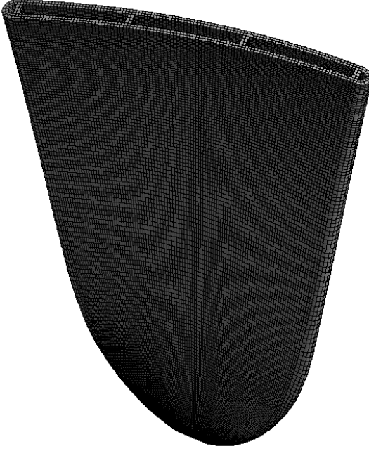
(b) Geometric tessellation of the reinforced blade profile
