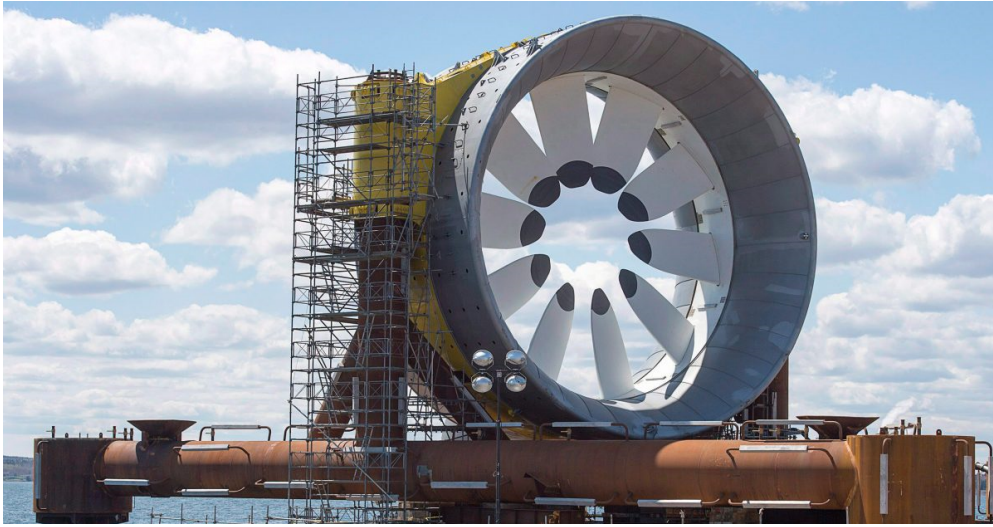
Figure 1: The 2 MW-rated OpenHydro ducted turbine. Adapted from [13], The Canadian Press/Andrew Vaughan, 2016.
