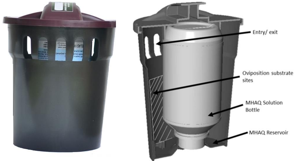
137 138 Figure 2. Mosquito Home System consisting of an oviposition substrate, MHAQ solution bottle 139 and MHAQ reservoir.
