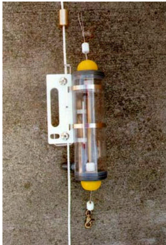
Figure 9. Vertical water sampler (Aquatic research webpage).
