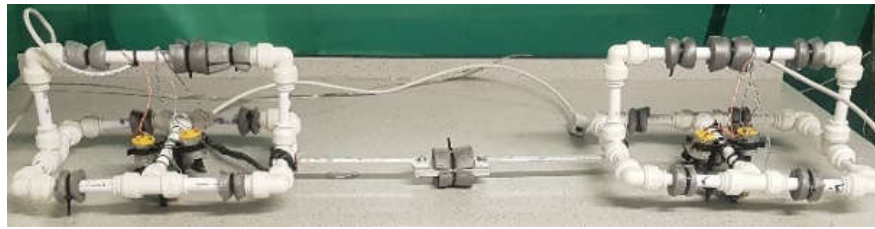
Figure 2. System of two Seaperch UUVs connected to a plated payload via plated manipulators (RCTS).
