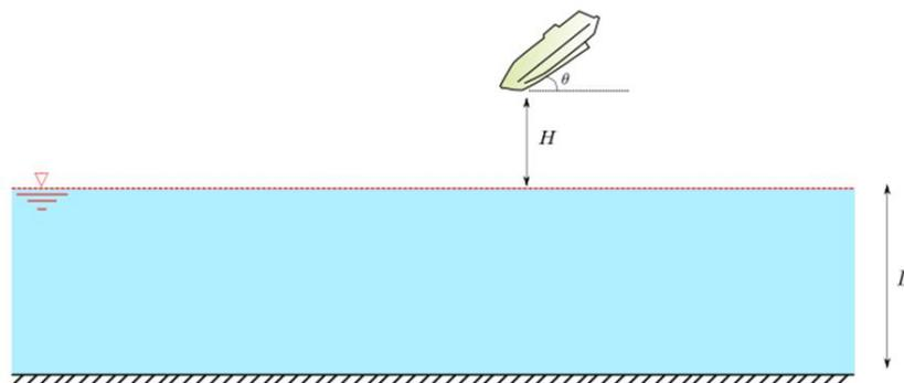
180 Figure 2: Schematic of the studied problem, showing a lifeboat is about to fall towards water surface
