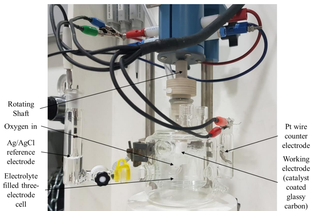
Figure 2.12: Photograph of the electrochemical cell used in the electrocatalytic testing of all materials.
