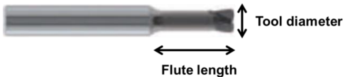
Figure 23: Schematic of the milling tool. Figure adapted from Dixi tools [171].
