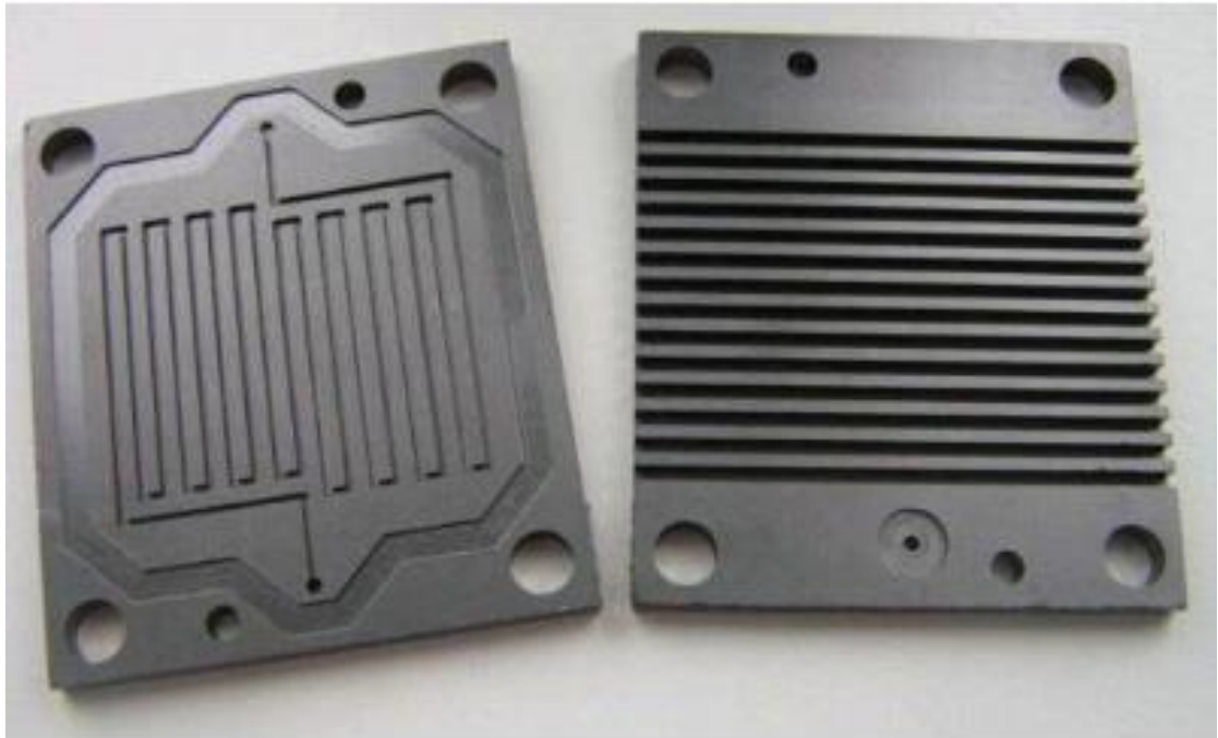
Figure 12: Graphite flow-field (bi-polar) plates for PEMFC. Figure adapted from [165].
