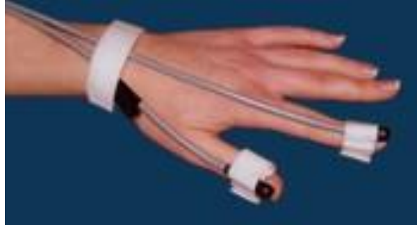
Figure 4.2: EM sensors were attached on nail beds of index finger and thumb.
