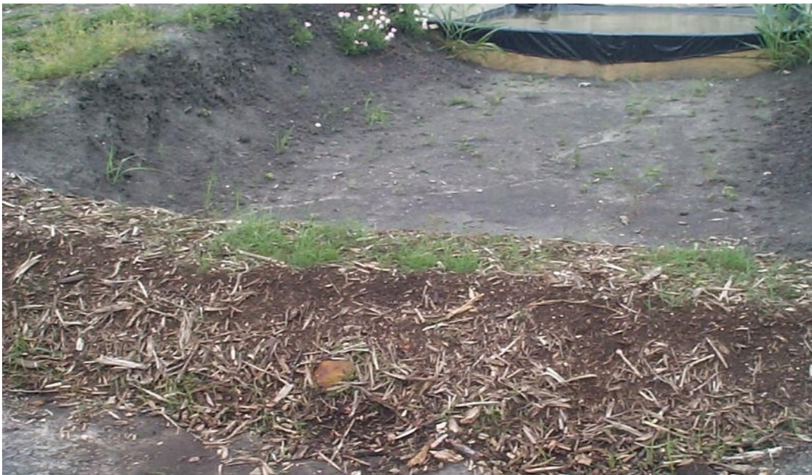
Figure 5.37 Dairy manure compost berm before starting the structural testing.
