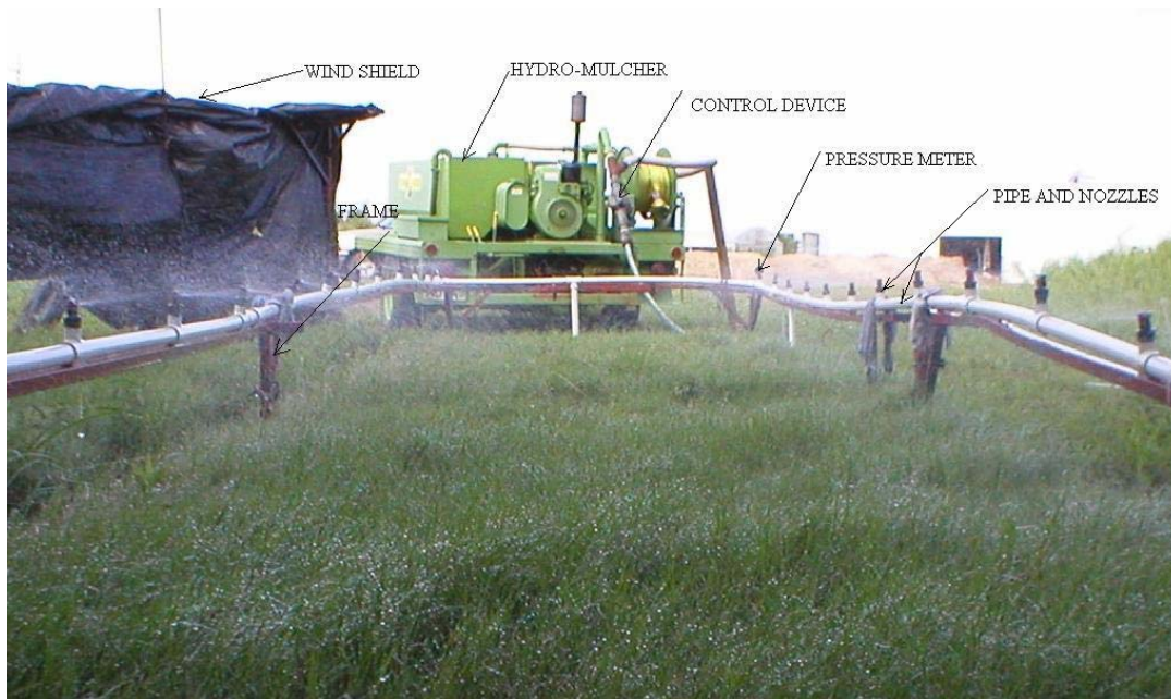
Figure 1 Rainfall Simulator
