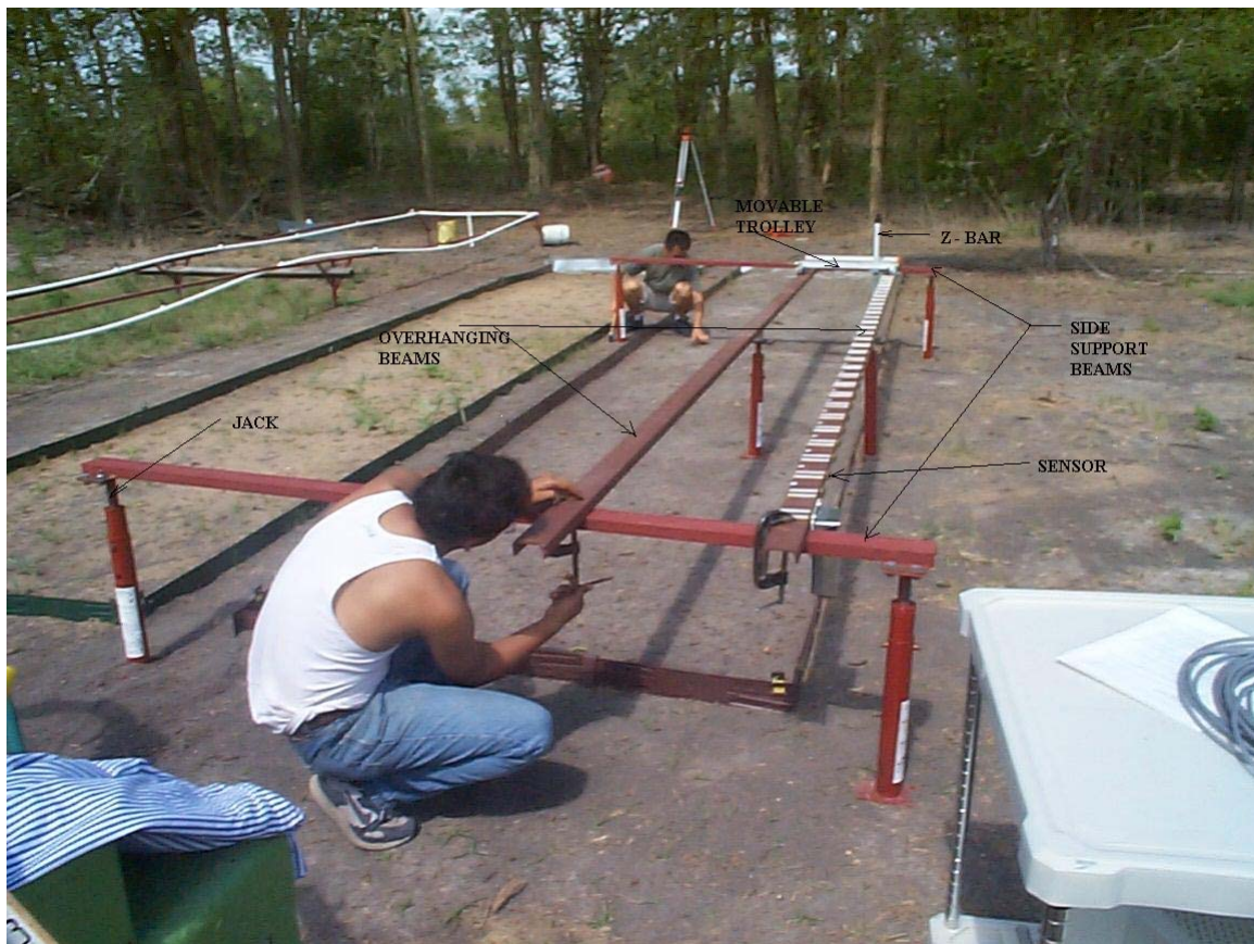
Figure 3 Microtopography Measurement System: Zimmometer
