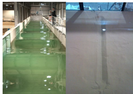
Fig. 1: The main channel of the Fast Flow Facility (left) and one of the initial trench profiles cut in sand (right)
