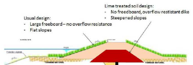
Figure 11: Typical profile for a flood controlled area embankment. Comparison between usual design and lime treated soil design.
