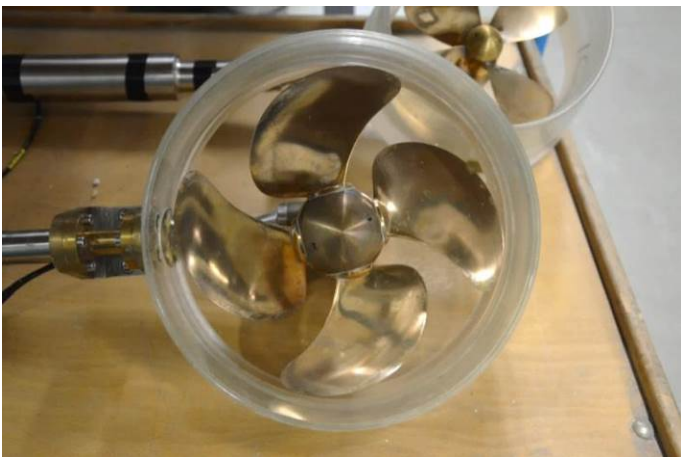
Figure 6. The scale model of the ducted propeller.
