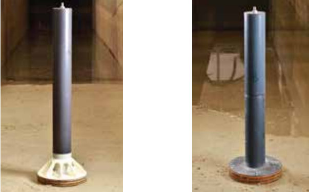
Figure 3: Models, left A and right C, used in the experimental analysis using variation height with respect to seabed.
