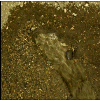
Figure 22. Failure of a shoulder made with suffusive alluvium caused by a concentrated leak.
