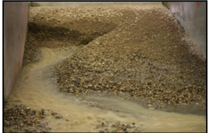
Test 3.1 2D flow - Failure. H_w=1.66 m h=1.5 m.
