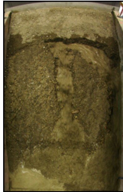
Figure 21. Photos of the failure of a shoulder made with alluvium caused by 2D flow.
