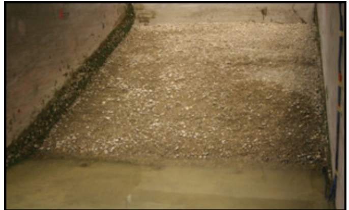
Test 3.5 Concentrated leak - No failure. H_w > 3 m h=1 m.
