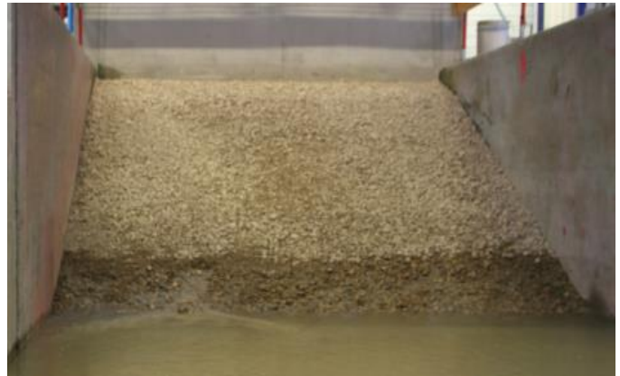
Test 3.1 2D flow erosion initiation H_w=0.9 m shoulder thickness h=1.5 m
