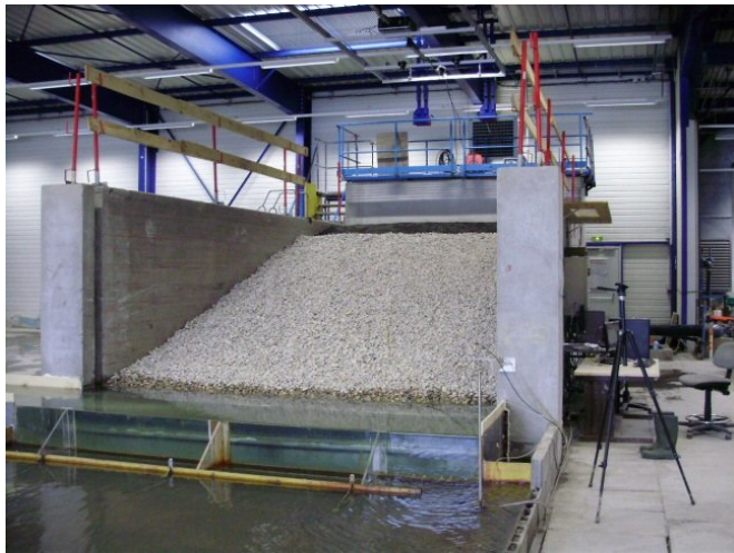
Figure 14. The dike studied in the second series of models (from Beguin 2011).
