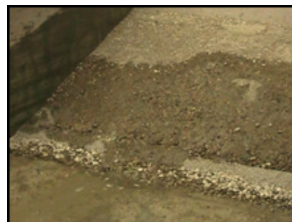
Figure 21. Photos of the failure of a shoulder made with alluvium caused by 2D flow.
