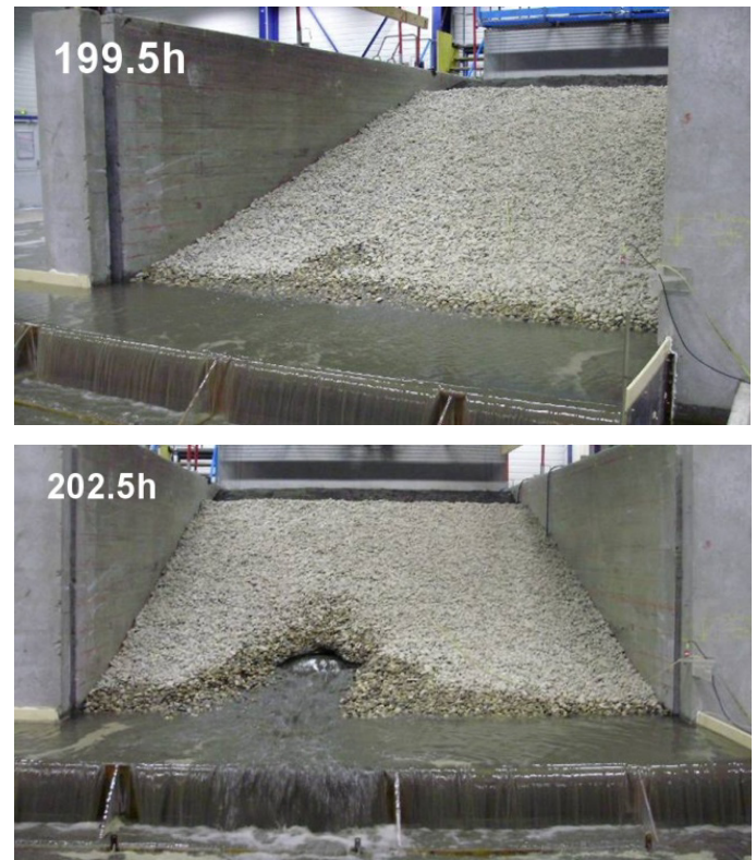
Fig.16: Piping exit in a levee suffering contact erosion (from Beguin, 2011).
