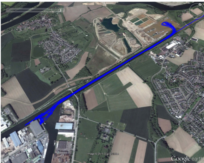
Figure 4. Measurement location with shiptracks of the barge (from AIS = Automatic Identification System) and the two turning points in the harbours. Source: Google earth.
