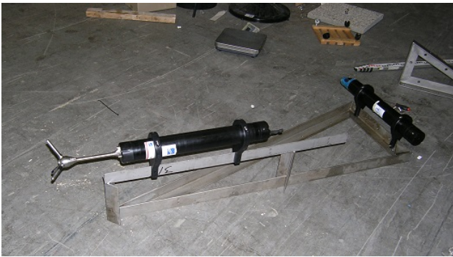
Figure 6. Bracket with Vector (looking sideways) and EasyQ (looking upward).
