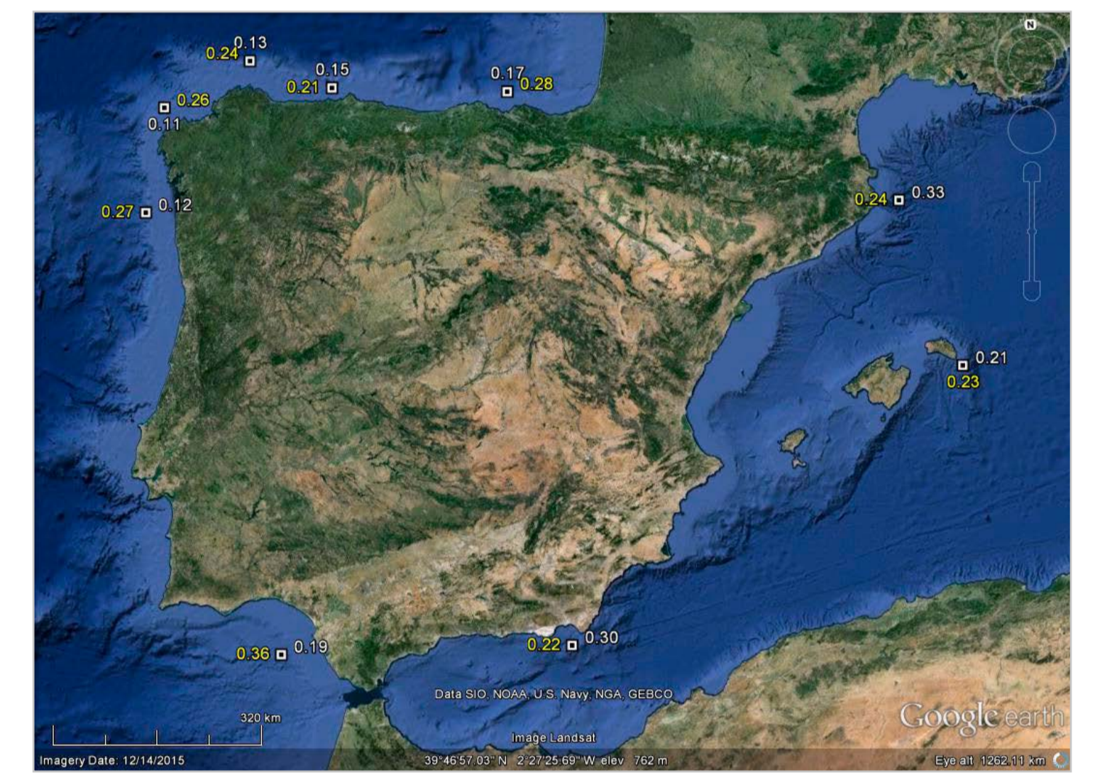
Scatter Index (standard deviation of error normalised by observed mean) in matched storm peaks, CFSR (white), ERA-Interim (yellow)
