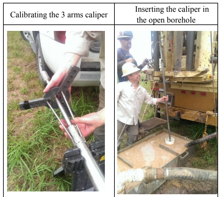
Figure 2. Borehole caliper for BET.
