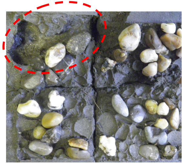
Figure 8. Interface between coarse soil and fine soil seen from below after the end of the test. The fine soil layer has been cut in four parts in order to be able to turn it back. Part of the gravel from the coarse soil has been removed and part of them is still in place. The pipe created by erosion is underline by a red circle
