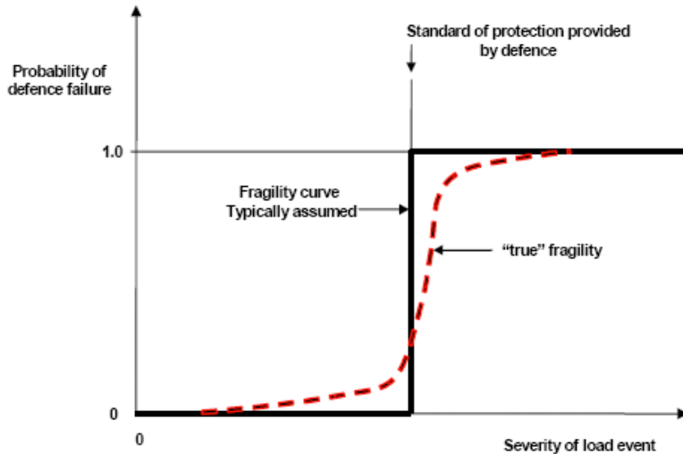
Figure 2: Example of a simplified and “true” generic fragility curve for flood defences
