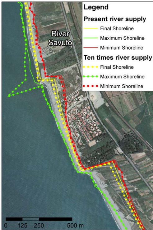
Figure 4: Sensitivity of the coastline to variation in sediment discharge from River Savuto, Italy.
