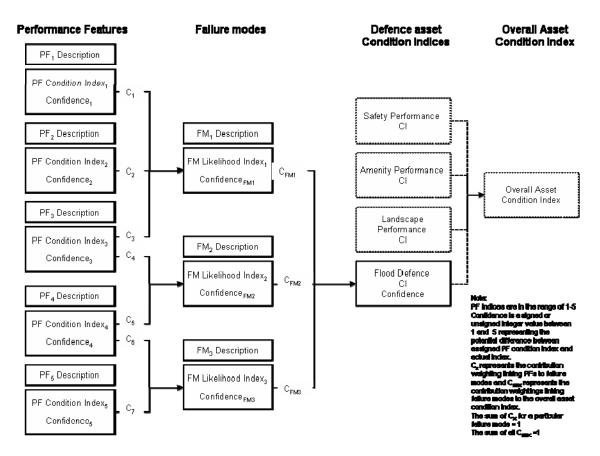
Figure 4 Condition indexing system for PAMS
