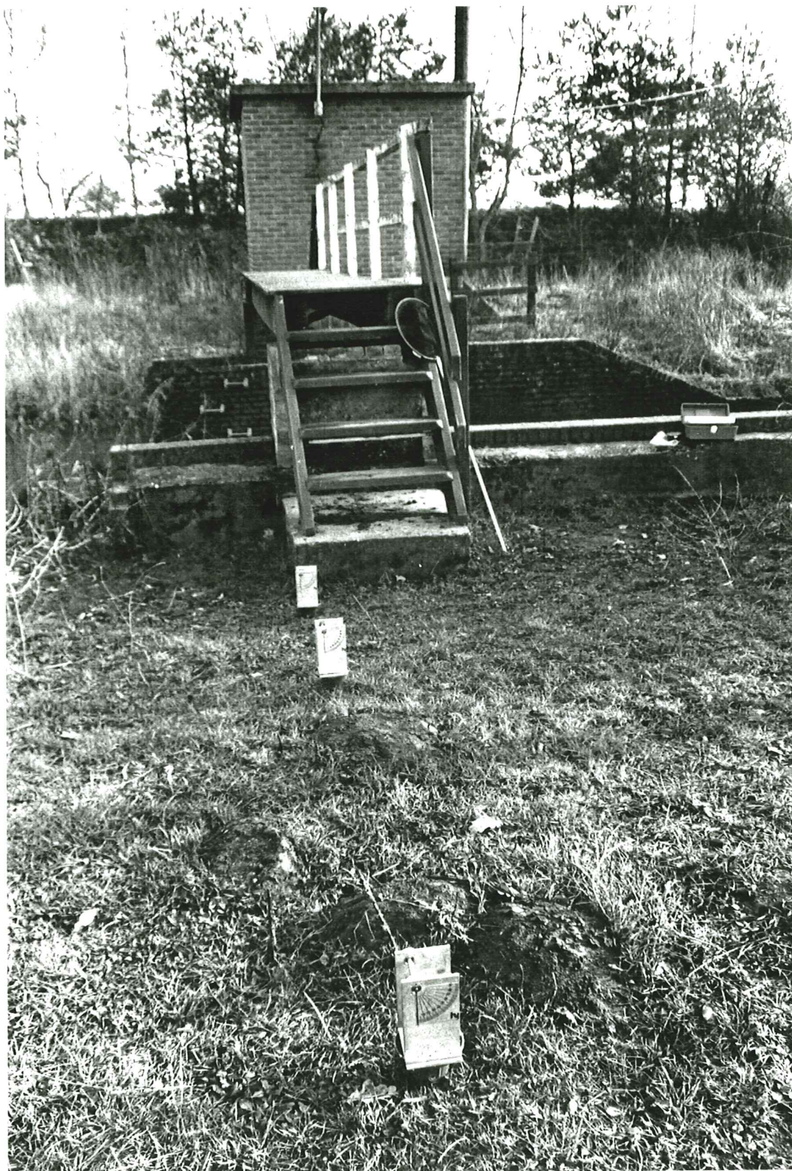
Plate 4 Peak velocity meters Nos 2 to 4 — right bank floodplain
