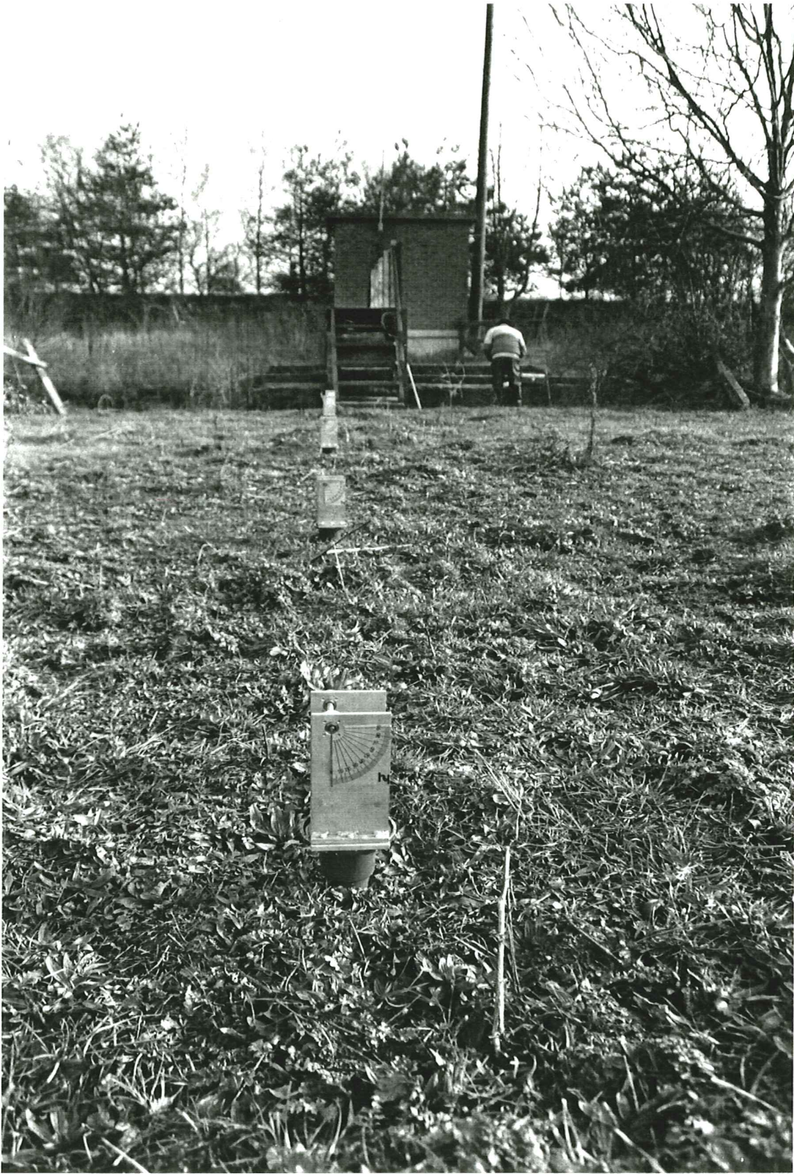
Plate 5 Peak velocity meters Nos 3 to 7 — right bank floodplain
