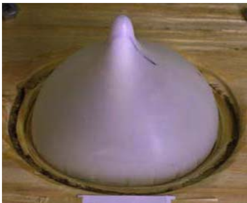
Fig. 34. Actual inflated profile for axis length 100mm and pressure of 2kpa.
