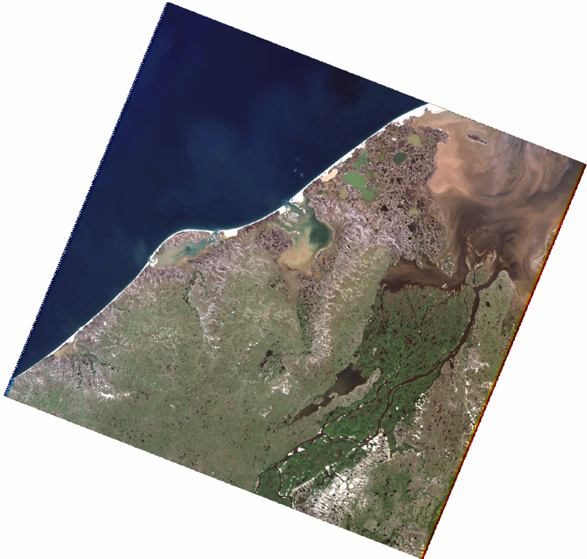
Figure 4.4. Landsat 7 ETM+ satellite sensor imagery used in the classification (displayed here with a RGB 321 (true colour) band combination) (170 x 183km).
