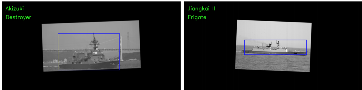
Figure 6. Examples of algorithm outputs on semi-labelled data during training (blue boxes and text are algorithm predictions). The depicted boxes were inferred by the algorithm, despite no ground truth bounding boxes being provided for these images.
