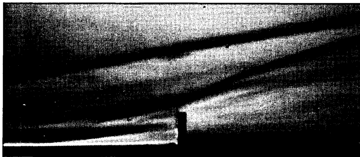
Figure 8.10 Schlieren image of blunt protuberance
